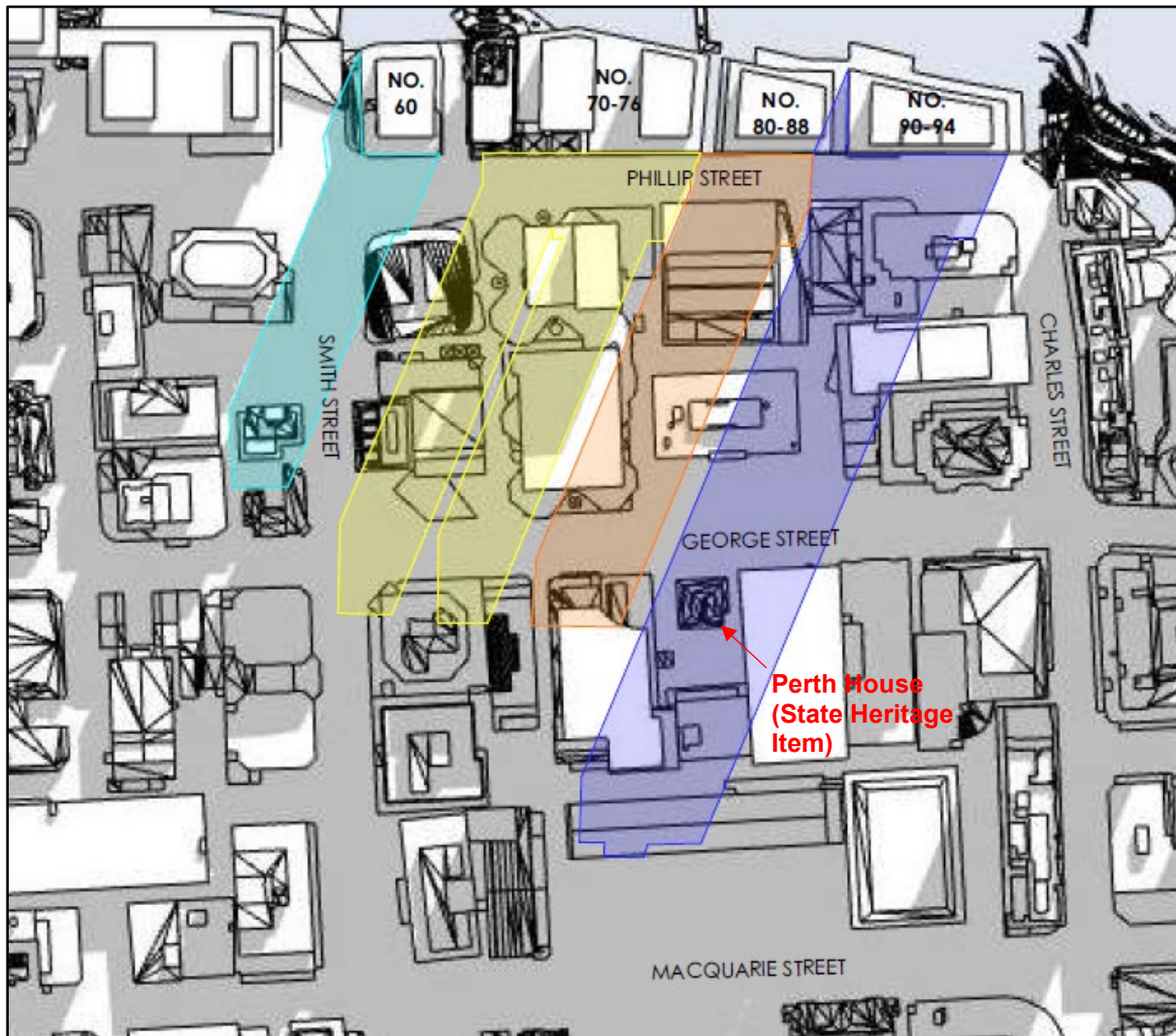
Figure 12: Extract from shadow diagrams showing shadows cast at 10.00am on 21 June (Source: Applicant's Reference Scheme – PTI Architecture). Shadow from subject site is shown in dark blue. Shadows from currently permissible development shown in grey shading.
